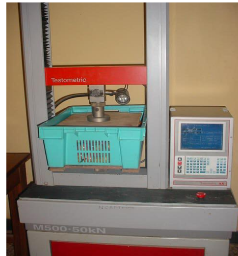
Fig. 1. Compression of tomatoes in plastic crate using Testometric Universal Testing Machine. (UTM).
